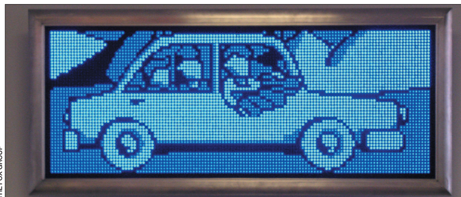
Fig. 4. Monochromatic 32 × 194 pixel sign, with dimensions of 0.45 × 1.2 m, using Fox Group's blue LEDs. The devices were not subjected to binning for color or forward voltage. Halftones were achieved by employing lower drive currents.
